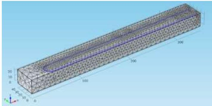
**Figure 2. Mesh of bridge deck and circulation fluid in 3D.**
