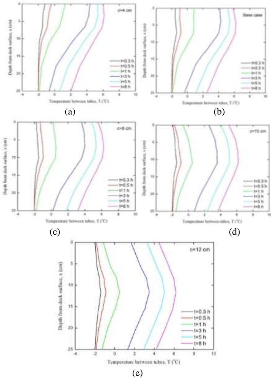
Figure 5. Temperature along the vertical section in between circulation pipes: (a)  $c=4$  cm; (b)  $c=6$  cm (Base case); (c)  $c=8$  cm; (d)  $c=10$  cm; (e)  $c=12$  cm.
