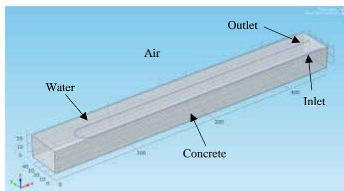
**Figure 1. Configuration of geothermal heated bridge deck.**
