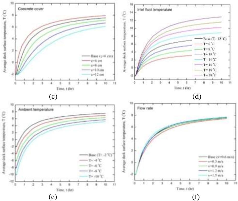
**Figure 3. Average temperature at top surface of bridge deck: (a) Pipe spacing; (b) Wind speed; (c) Concrete cover; (d) Inlet fluid temperature; (e) Ambient temperature; (f) Flow rate.**
