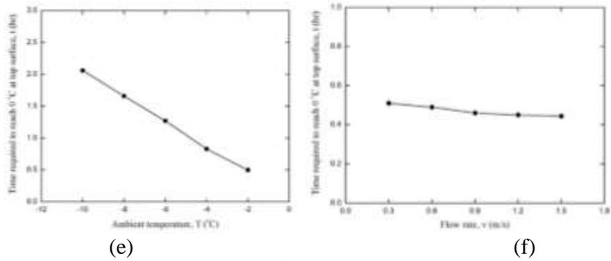
Figure 4. Time required to reach 0°C at top surface of bridge deck: (a) Pipe spacing; (b) Wind speed; (c) Concrete cover; (d) Inlet fluid temperature; (e) Ambient temperature; (f) Flow rate.
