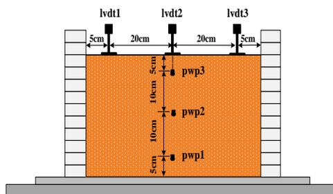
Figure 4. Schematic diagram of transducer arrangement.
