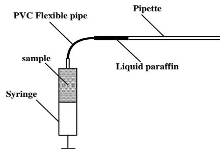
**Figure 2. Schematic diagram of gas measurement device.**
