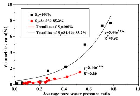
Figure 9. Plot of volumetric strains against average pore water pressure ratios.
