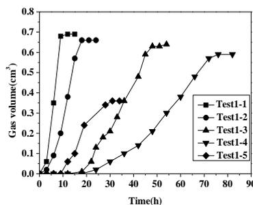
**Figure 6. Gas generation curve with different temperatures.**
