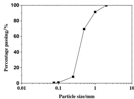
**Figure 1. Particle-size distributions curve of sand sample.**
