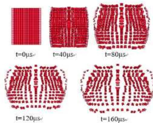
Figure 5. The physical process of flight of fragment.
