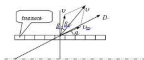
Figure 3. Scattering angles of fragments of the dynamic explosion.
