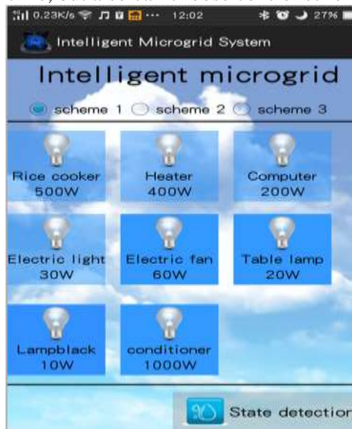
Figure 4. Intelligent microgrid control.
