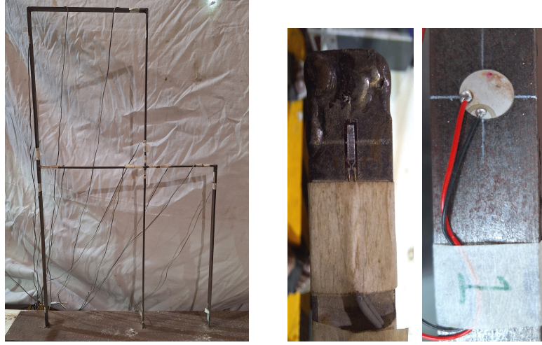
Figure 2. (left) Full experimental setup, (right) Enlarged image of employed strain gauge and PZT patch.
