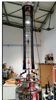
Figure 4: FBGS stand-alone thermal cycling tool.
