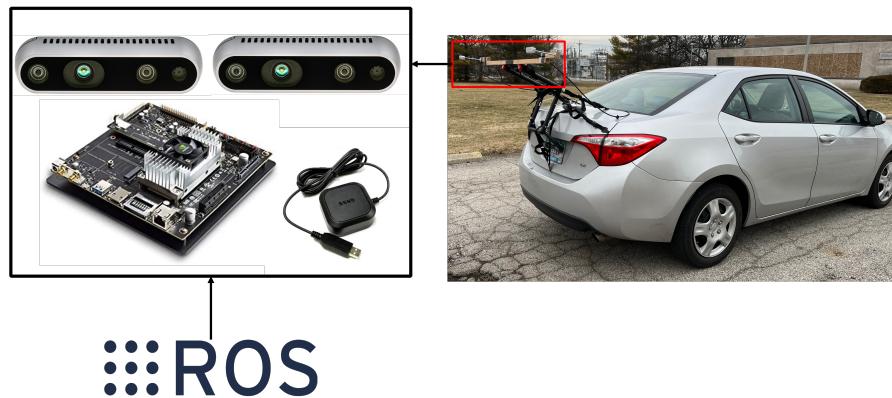
Figure 1. Data collection system configuration. The proposed data acquisition system includes two RGB-D sensors, one edge computing device, and a GPS sensor. All sensors are integrated through Robotic Operating System. The system can be easily mounted on a bike rack at the trunk.
