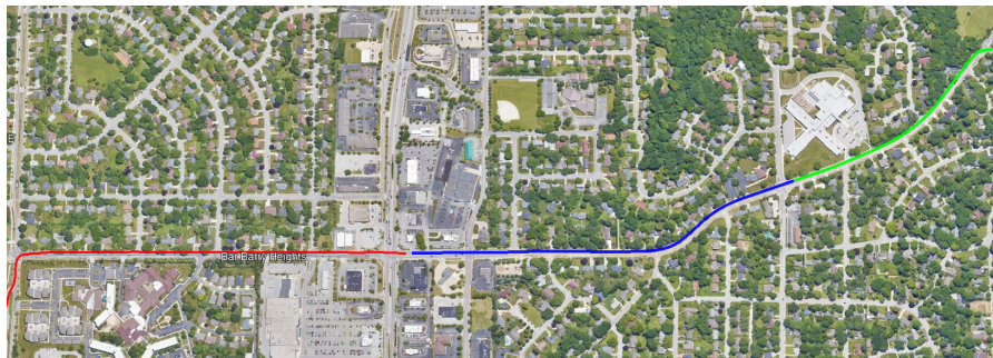
Figure 4. An example of data collection route. The color of the path corresponds to distinct conditions of the PASER, where red signifies the poor condition, blue denotes the fair condition, and green designates the good condition. The total length of this route amounts to 1.4 miles.
