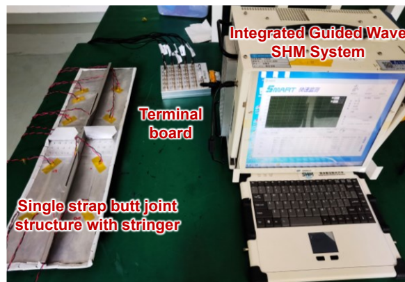
Figure 2. Test system for Experiment on guided wave propagation characteristics.
