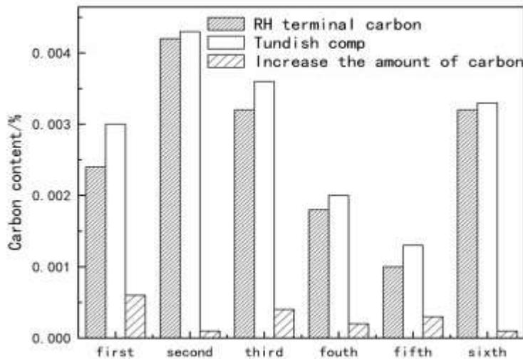
Figure 1. Carbon content differences between RH ending and tundish/%.
