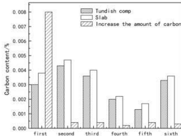
Figure 2. Carbon content differences between tundish and casting/%.
