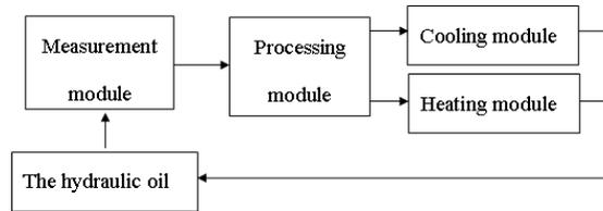
Figure 1. The oil temperature automatic control system for the overall scheme of the control block diagram.
