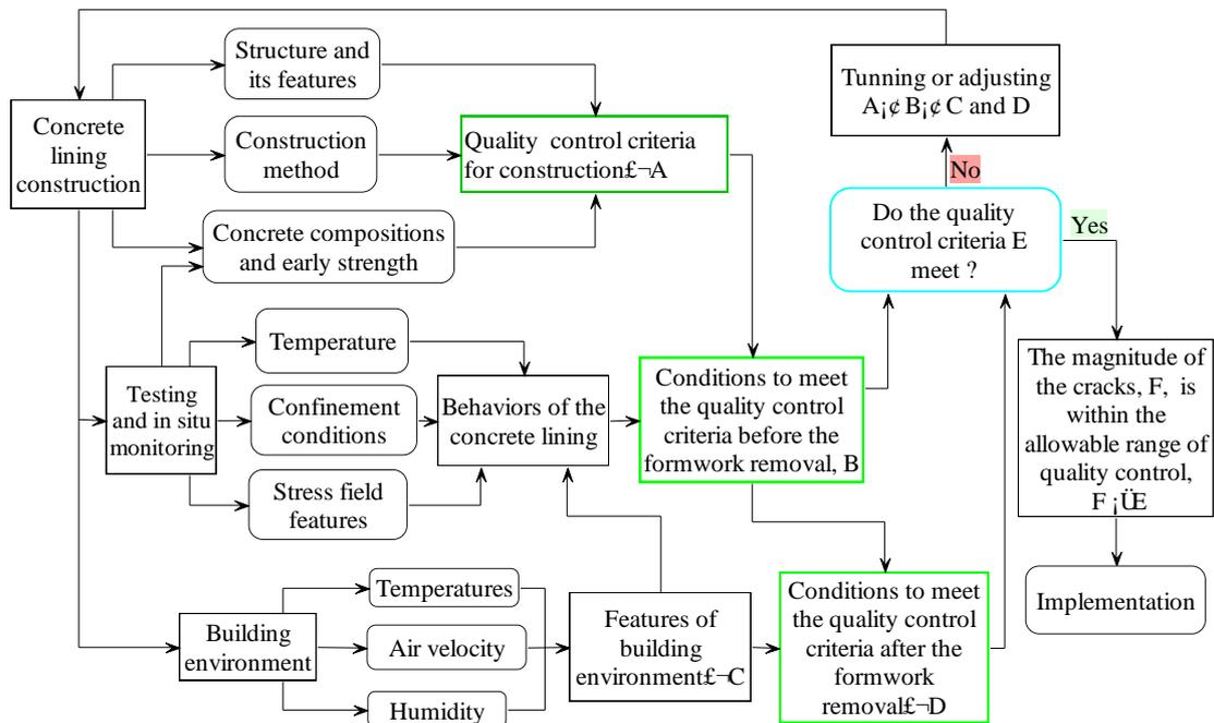
Figure 2. Key Information related to the cracking control of the tunnel concrete lining and sharing in procedure.
