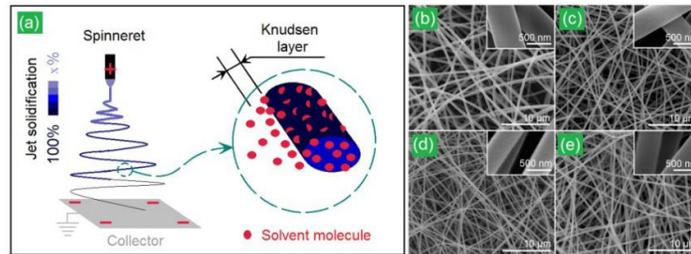
Figure 4. The Utilization of Scientific Phenomena as Teaching Materials in Explaining the Solidification of Fluid Jets during the Bending and Whipping Processes. (a) A Schematic Diagram about the Knudsen Layer on A Fluid Jet in the Instable Region; (b) to (e) are SEM Images of the Solidified Products Fabricated under Temperatures of 20, 30, 40 and 50 °C, respectively [22].
