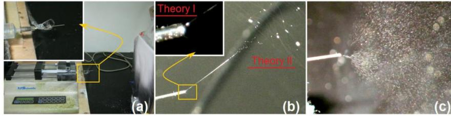
Figure 1. Implementation and Theories about the EHDA Processes. (a) The Typical Components of an EHDA System, the Inset Shows the Connection between the Power Supply with the Working Fluids; (b) A Typical Working Process of Electrospinning, During Which Two Related Theories Are Involved, the Inset Shows an Enlarged Taylor Cone ; (c) A Similar Electrospaying Process.
