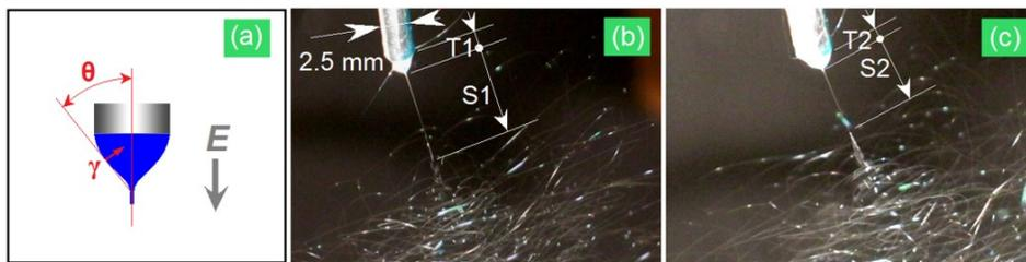
Figure 3. The Utilization of Scientific Phenomena as Teaching Materials in Explaining the Formations of Taylor Cones and Straight Fluid Jets. (a) A Schematic Diagram about the Taylor Cone; (b) A Digital Picture of the Taylor Cone Initiated at A Working Distance of 20 cm; and (c) A Digital Picture of the Taylor Cone Initiated at A Working Distance of 12 cm.
