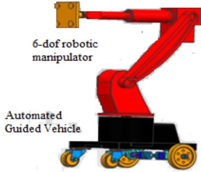
Figure 1. Robotic tiling machine.
