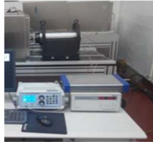
Figure 6. Experiment platform of variable preload device.
