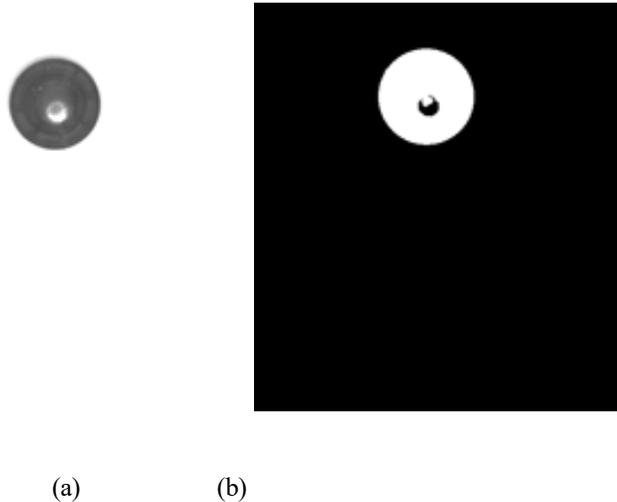
Figure 3. Background removal. (a) Origin image; (b) Background removed image.
