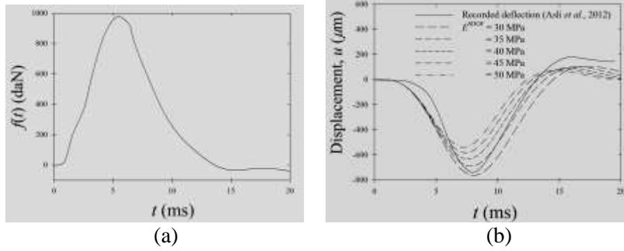
**Figure 5. (a) The applied load pulse  $f(t)$  by FWD test on clayey soil and (b) displacement profiles from the recorded field data (Asli *et al.*, 2012) and the dynamic SDOF model for clayey soil.**
