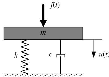
**Figure 2. Schematic illustration of dynamic single degree of freedom (SDOF) model.**
