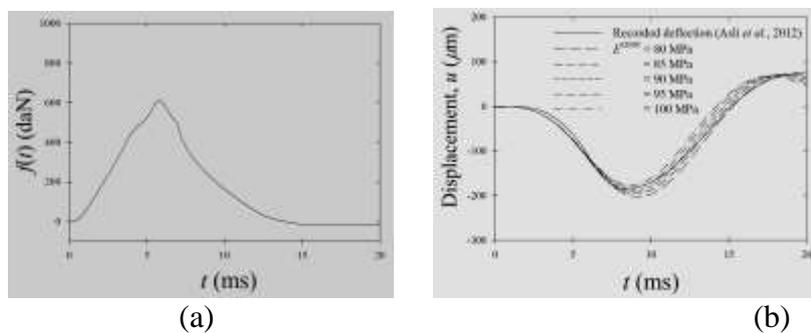
**Figure 4. (a) The applied load pulse  $f(t)$  by FWD test on CCA soil and (b) displacement profiles from the recorded field data (Asli *et al.*, 2012) and the dynamic SDOF model for CCA.**
