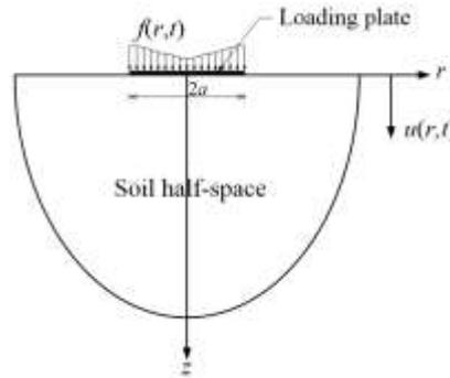
**Figure 3. Schematic illustration of dynamic half-space model considered in the present study.**
