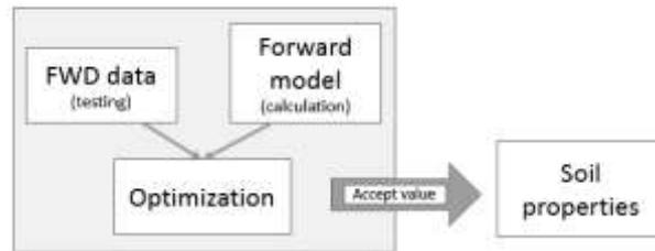
**Figure 1. Falling weight deflectometer (FWD) backcalculation process.**
