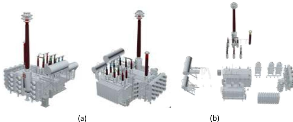
**Figure 4.** Main transformer thumbnail. (a) Panoramic view of main transformer; (b) Main components of main transformer.
