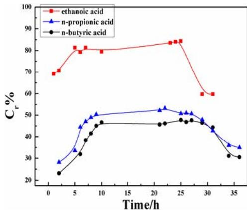
Figure 6. The relationship between  $C_r$  of PGA treated with monoacid and time.
