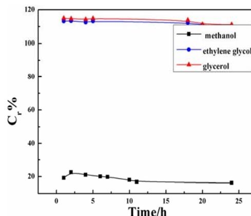
Figure 5. The relationship between  $C_r$  of PGA treated with polyalcohol and time.
