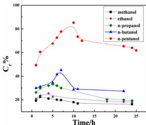
Figure 4. The relationship between  $C_r$  of PGA treated with monoalcohol and time.
