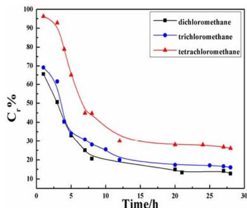
Figure 3. The relationship between  $C_r$  of PGA treated with chlorinated methane and time.
