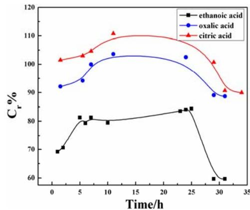
Figure 7. The relationship between  $C_r$  of PGA treated with polyacid and time.
