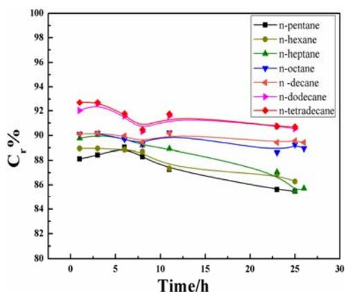
Figure 2. The relationship between  $C_r$  of PGA treated with n-alkane and time.
