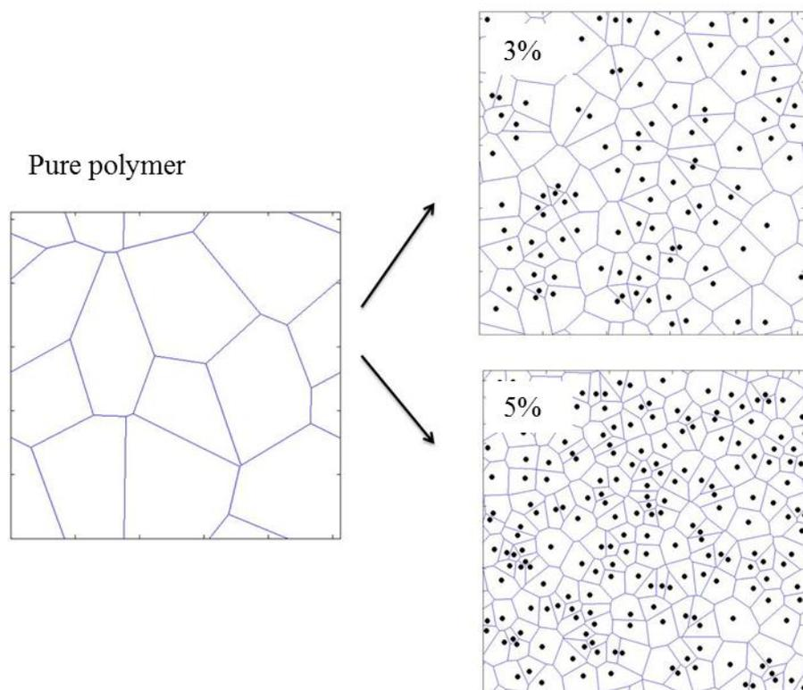
**Figure 1. Schematic illustration of change in voronoi size after adding nanoparticles to Semicrystalline polymer (RVE models generated using MATLAB)**
