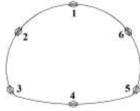
Figure 2. Diagram of layout of strain gauges.
