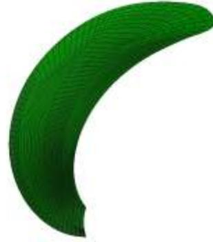
Figure 2. Blade mesh of DTMB 4384.
