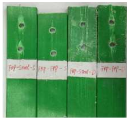
Figure 3. The Failure Mode of Bolt connection. Figure 4. The Failure Mode of mixed connection.
