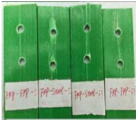
Figure 3. The Failure Mode of Bolt connection. Figure 4. The Failure Mode of mixed connection.
