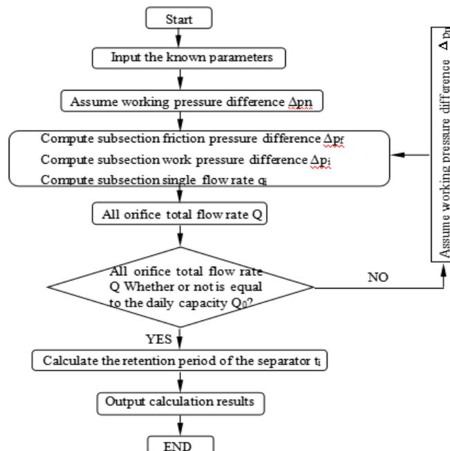
Figure 4. Computing diagram of residence time.
