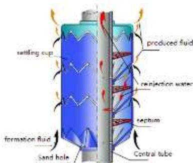
Figure 1. Oil-water separator.
