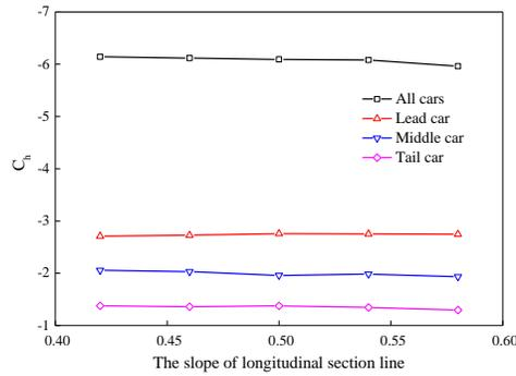
Figure 9. The lateral force of different trains.
