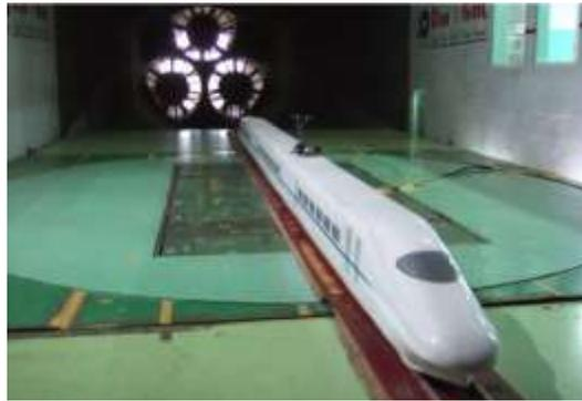
Figure 6. The wind tunnel test.
