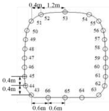
Figure 10. The measuring points of the middle car.
