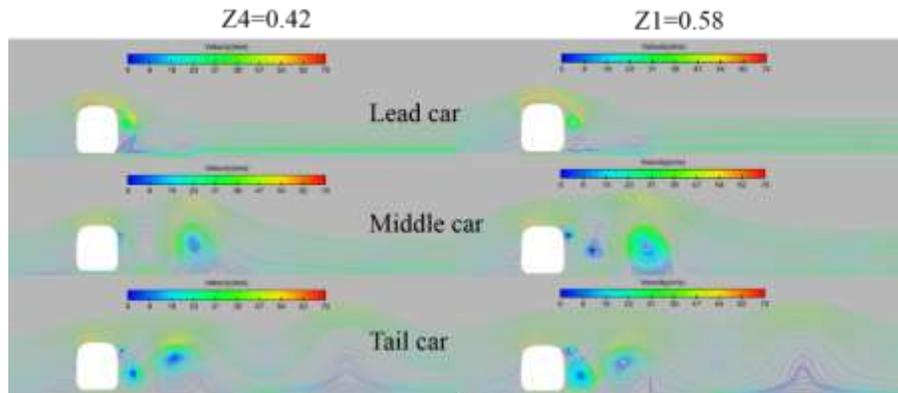
Figure 12. The streamline diagram around the train.
