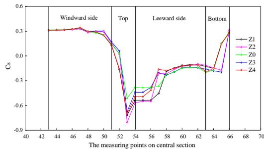
Figure 11. The surface pressure coefficient of intermediate section of different trains.
