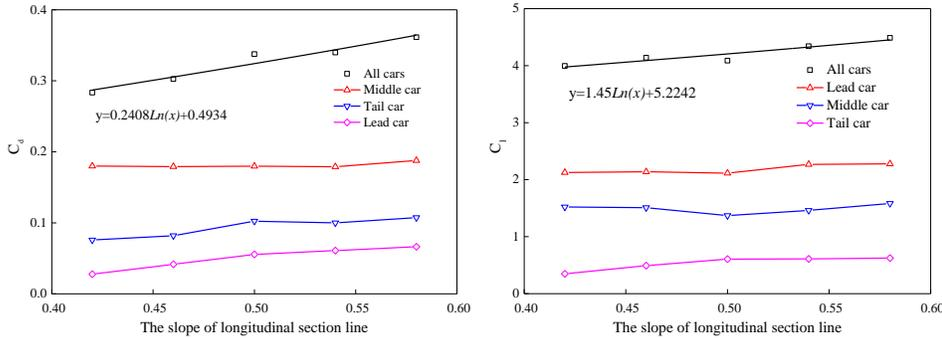
Figure 7. The drag coefficient of different trains. Figure 8. The lift force of different trains.
