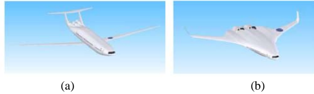
Figure 3. (a) Double-bubble (D8 Series) and (b) hybrid wing body (H3 Series) conceptual aircraft [8][9].
