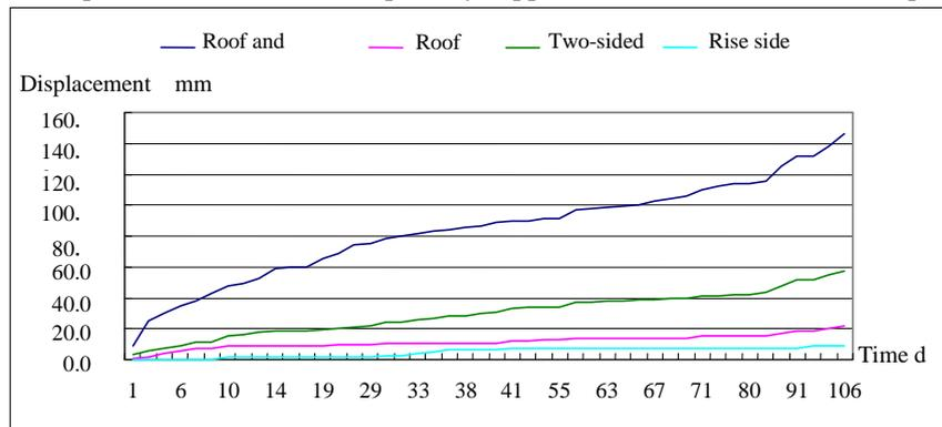
(b) Displacement curve chart of test zone surface for No.1411 up drift
