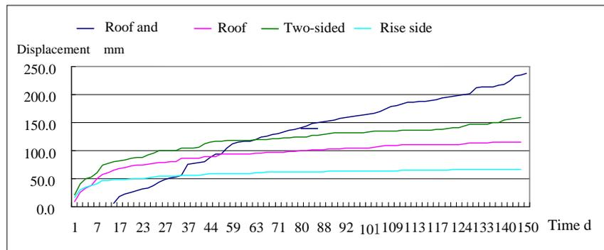
(a) Displacement curve chart of primary support zone surface for No.1411 up drift
