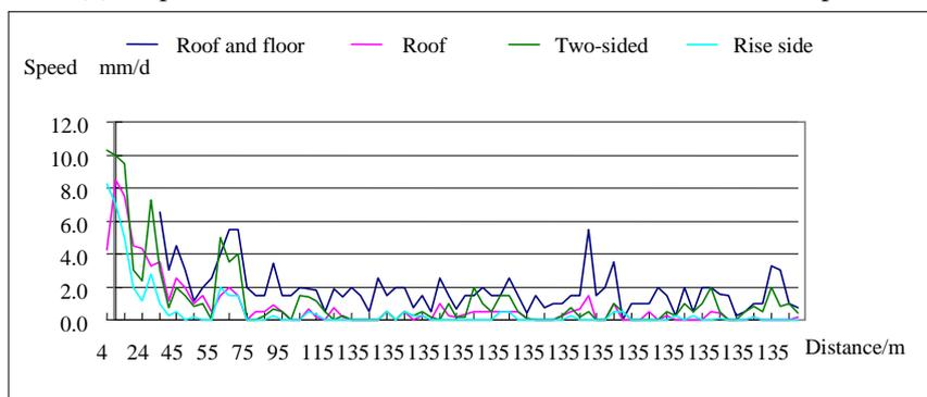
(c) Displacement velocity curve chart of primary support zone surface for No.1411 up drift
