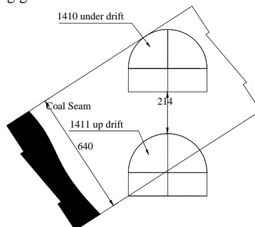
Figure 2. Roadway layout schematic.
