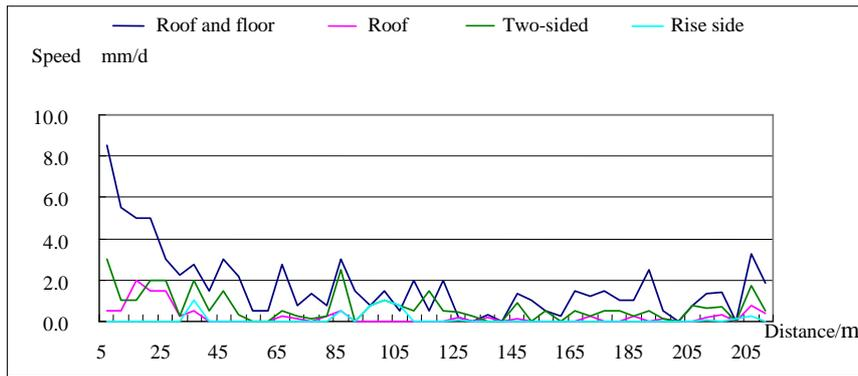
(d) Displacement velocity curve chart of test zone surface for No.1411 up drift
