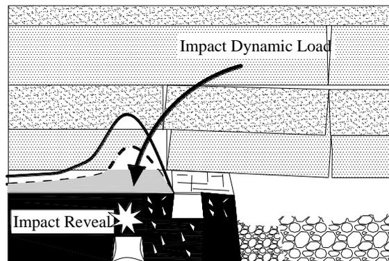
Figure 1. The rock burst occurrence in No.1411 up drift by "the principle of superposition movement".
