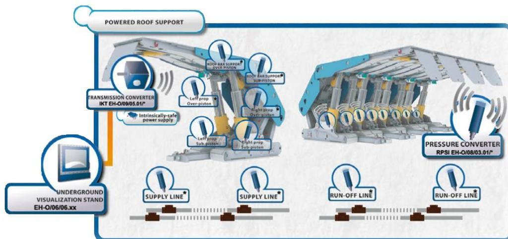
Figure 1. EH-PressCATER wireless monitoring system [5].
