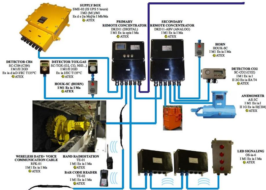
Figure 2. DPS11 mine telemonitoring system diagram [15].
