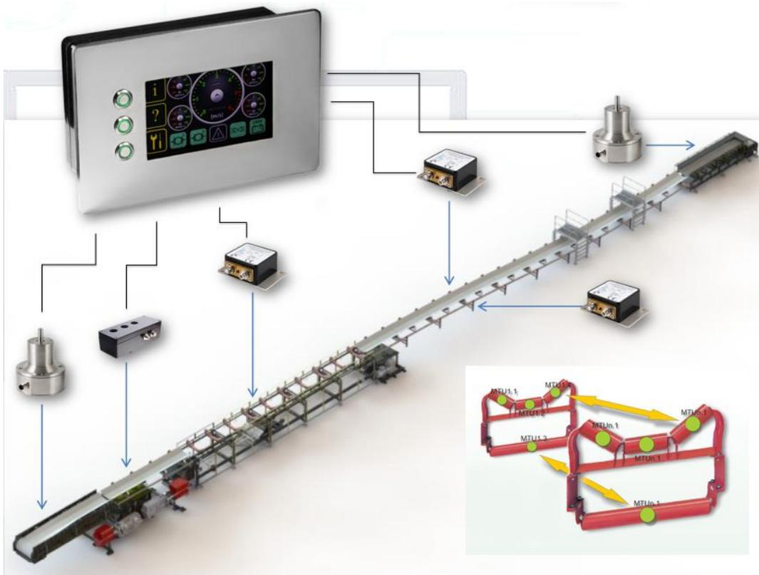
Figure 4. Example of implementation of the SSKIR protocol in sensory network of belt conveyor rollers [8].
