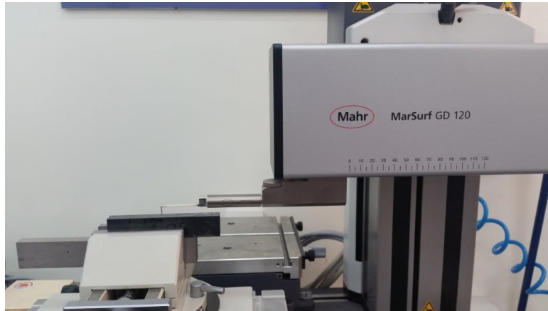
Figure 2. A sample photograph of the roughness measurement.
