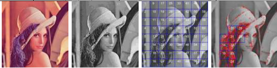
(a) Original image (b) Luminance image (c) Labels of the blocks (d) Ten effective blocks
